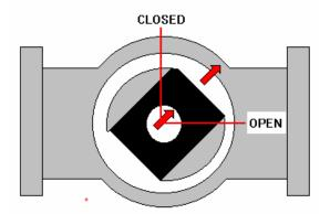
After all valves have been turned ½ open/closed the VCT shall approve the start-up of the hydrostatic test pumps. Pressure will be taken to 50% of MOP, the pumps shall be stopped and every valve, flange and fitting shall be visually inspected for signs of leakage. After all visible leak points have been eliminated the pumps shall be started and the pipeline taken to full test pressure.
