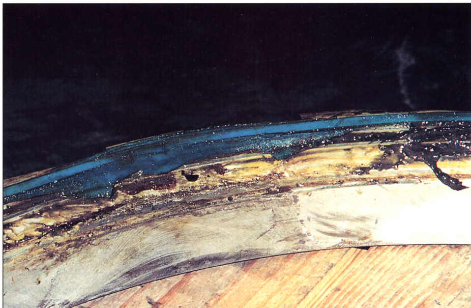
Photograph of a seat ring from a large-diameter welded body ball valve. The seat ring insert has obviously melted. This damage occurred during construction when the valve pup was pre-heated prior to welding the valve into the pipeline. Notice what appears to be metal shavings embedded into the insert. The shavings may have been introduced as a result of a hot tapping exercise some distance upstream of the valve site.
