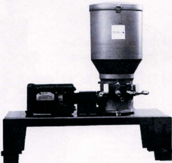
Automatic valve lubricator developed by Nova Corp. of Alberta has been in service for more than 3½ years.
