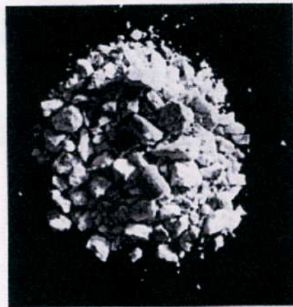
Residue from stick type lubricants that was scraped from valve grooves.
